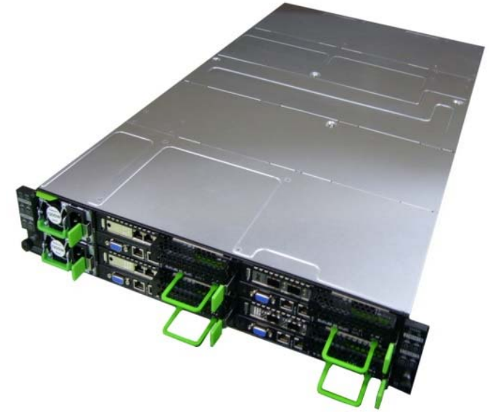
Chassis with 8 nodes, 2U size
